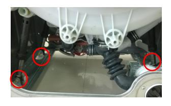
20. **Undo the tub assemble**I.Undo the rear cover, top cover, control panel, front panel, top
