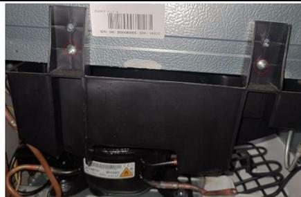
2) Replace the drain tray, the reverse process can complete installation.
