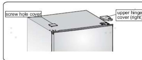
3. Remove the three screws as follow diagram. Lift the right upper hinge part.
