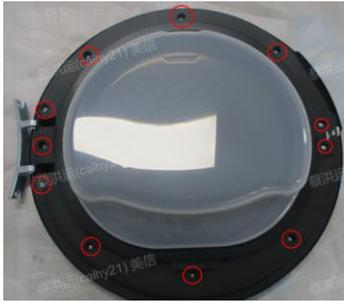
A top-down photograph of the inner ring, showing 11 screws marked with red circles for removal.                                                          |
