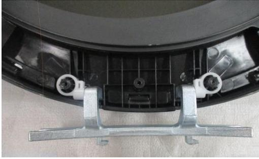
A close-up photograph of the door hinge mechanism being removed from the door.                                                                        |
