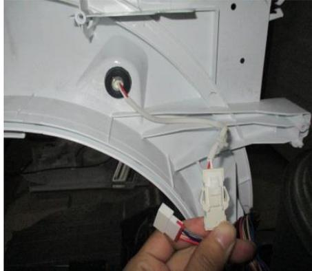
A close-up photograph of a person's hands pulling out a white plastic wire terminal from the front support assembly. The terminal is connected to a small lamp. The background shows the white plastic housing of the assembly.                                      |
