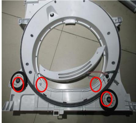
A photograph showing the front support assembly with two screws on the humidity sensor support circled in red. The assembly is shown from a slightly elevated front perspective.                                                                                    |
