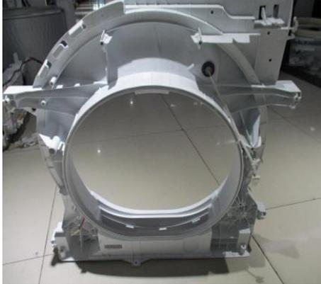
A photograph showing the front support assembly with the felt ring seal removed. The circular opening is now empty. The two wheels at the bottom are still attached. The assembly is shown from a slightly elevated front perspective.                              |
