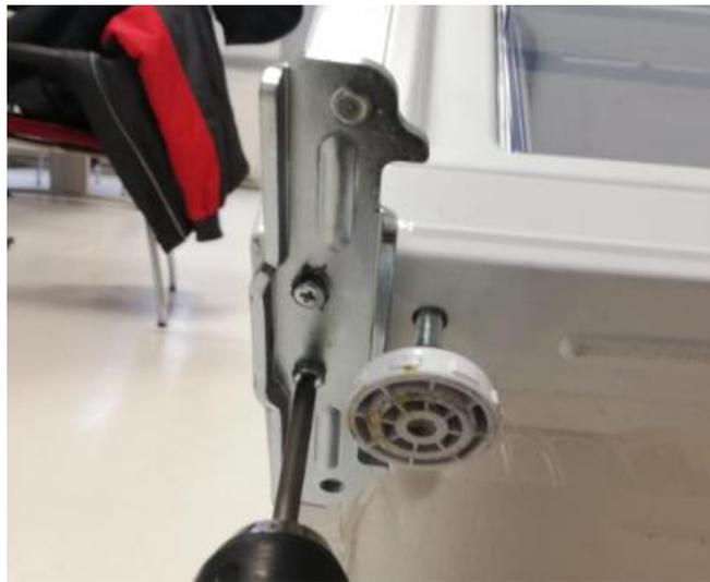
**REMOVE THE LOWER HINGE BEARING OF THE FF COMPARTMENT DOOR**
