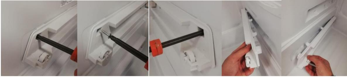
After the glass shelves are pulled forward as shown in the images below, the rear profile is lifted to be removed from the form on the body and pulled out first.
