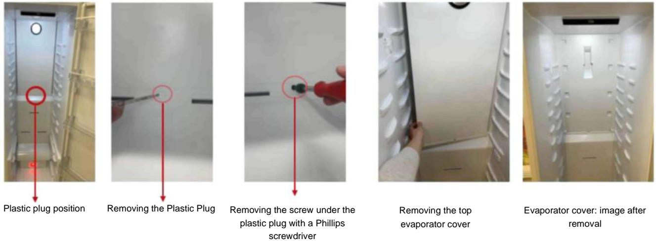
Picture 2: Removing the top evaporator cover.
