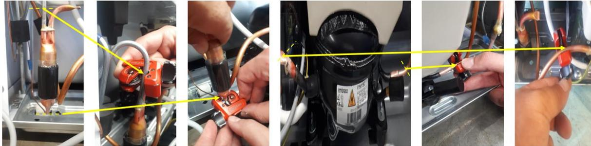
Picture 10: Cutting compressor and dryer pipes
