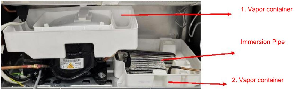
Picture 7: Vapor container & Immersion pipe
