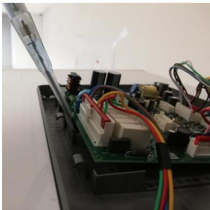
The Wi-Fi / humidity sensor cover is removed as shown in the picture.
