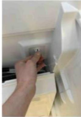
Removing the defrost heater cable from the socket
