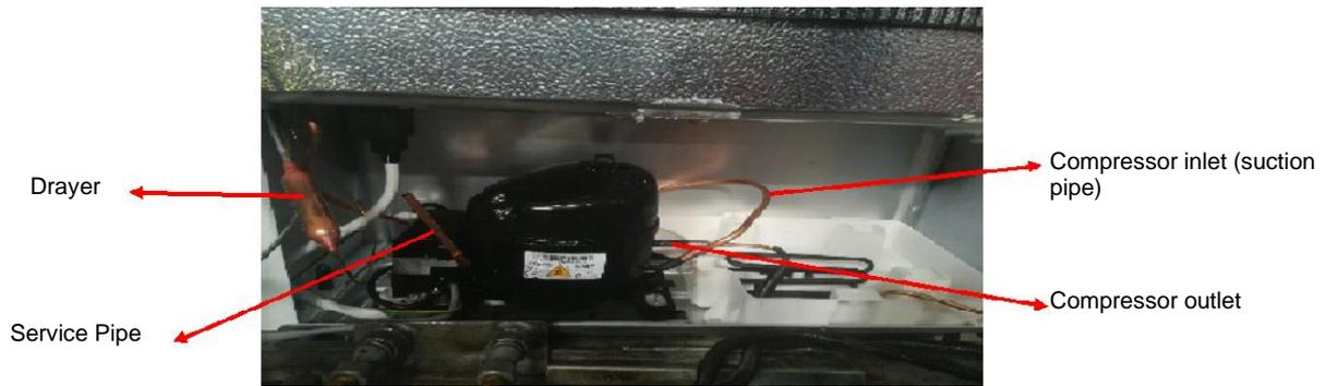
Picture 9: Pipes related to compressor and dryer
