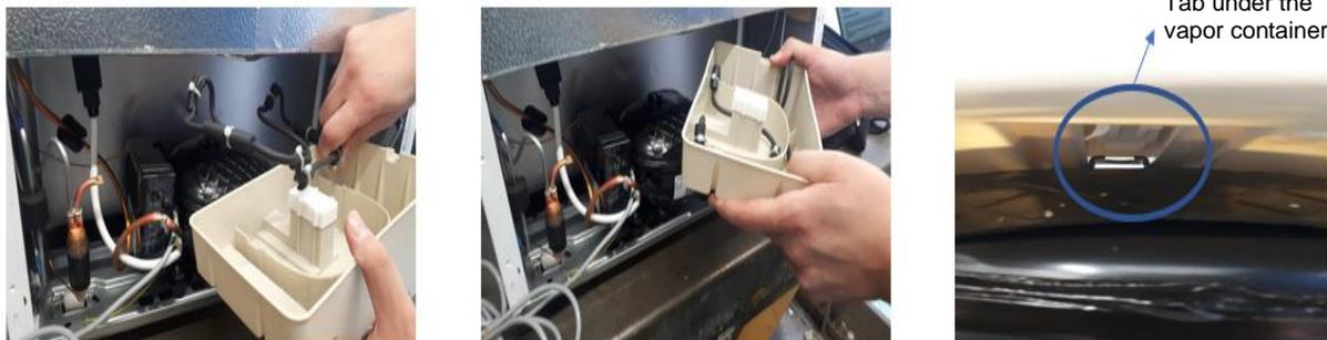
Picture 8: Removing and installing the vapor container
