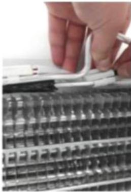
Removing the evaporator temperature switch
