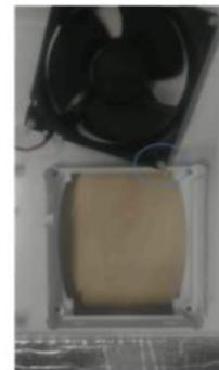
Pull the silicone connections on the other surface and remove the fan from the back cover.
