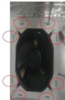
Use a flat screwdriver to disconnect the claw connections.
