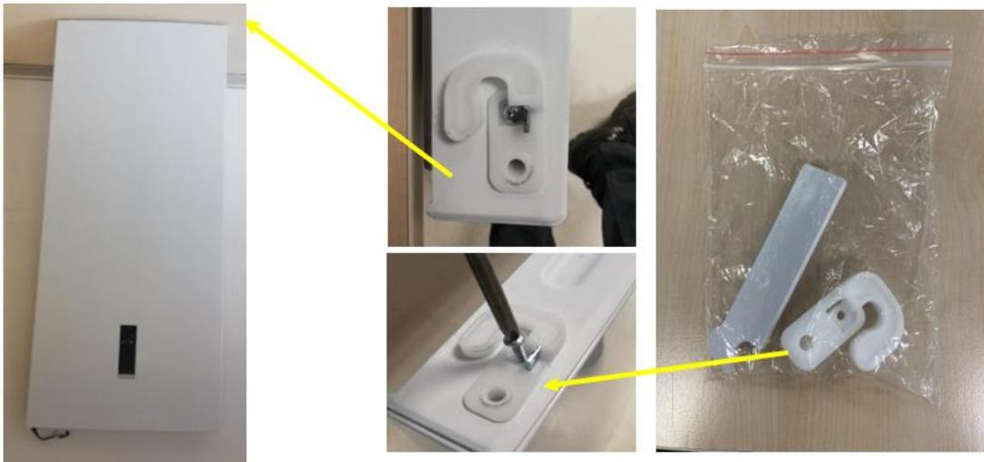
**REMOVE THE DOOR CABLE SLOT COVER**
