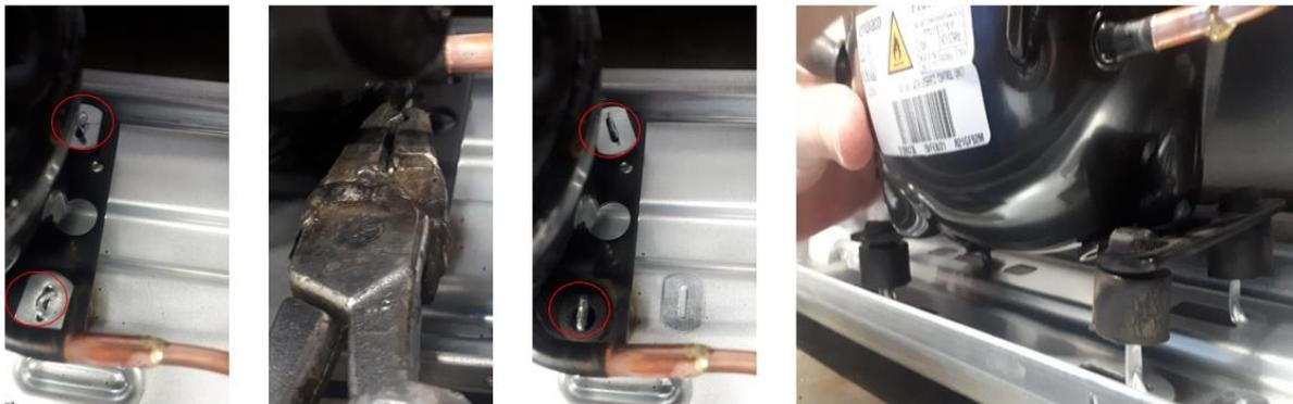
Picture 11: Removing the compressor foot stabilizers
