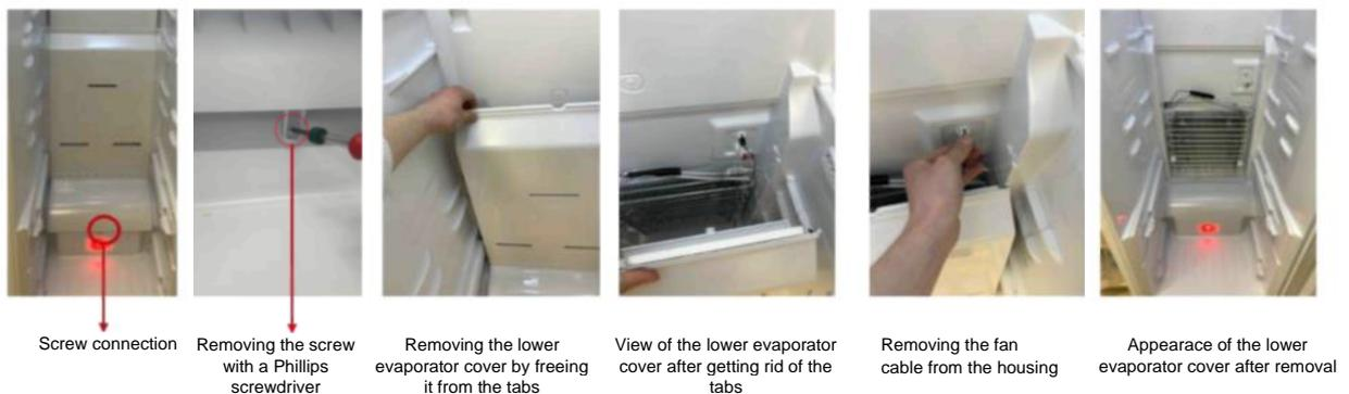
Picture 3: Removing the bottom evaporator cover.
