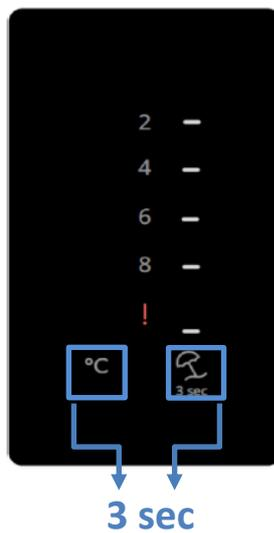
All the LEDs will alternately turn on for 0.5 seconds and turn off for 0.5 seconds.
