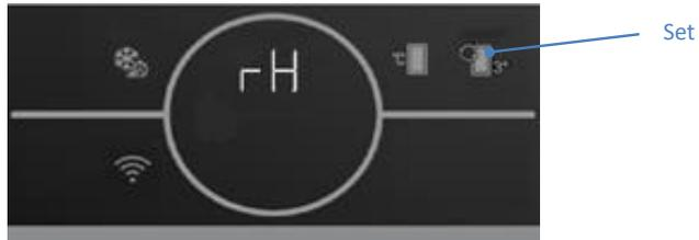
When the Set and quick freeze keys are pressed shortly together, the step progresses to driving the SC selected components.
