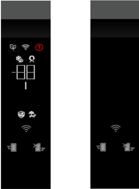
When the Vacation key is pressed once, the display is shown, if it is pressed once more, the version-revision information of the control card is shown.
