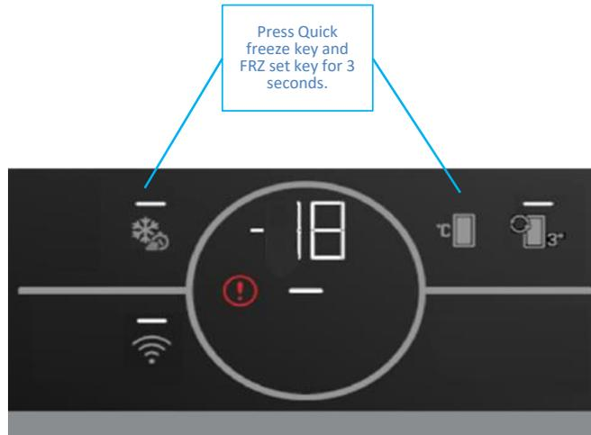
Press the Quick Freeze key once on the PS screen to confirm the PS-0 and enter the service test.
